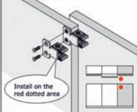
Install inner door stopper for 3-door-type
